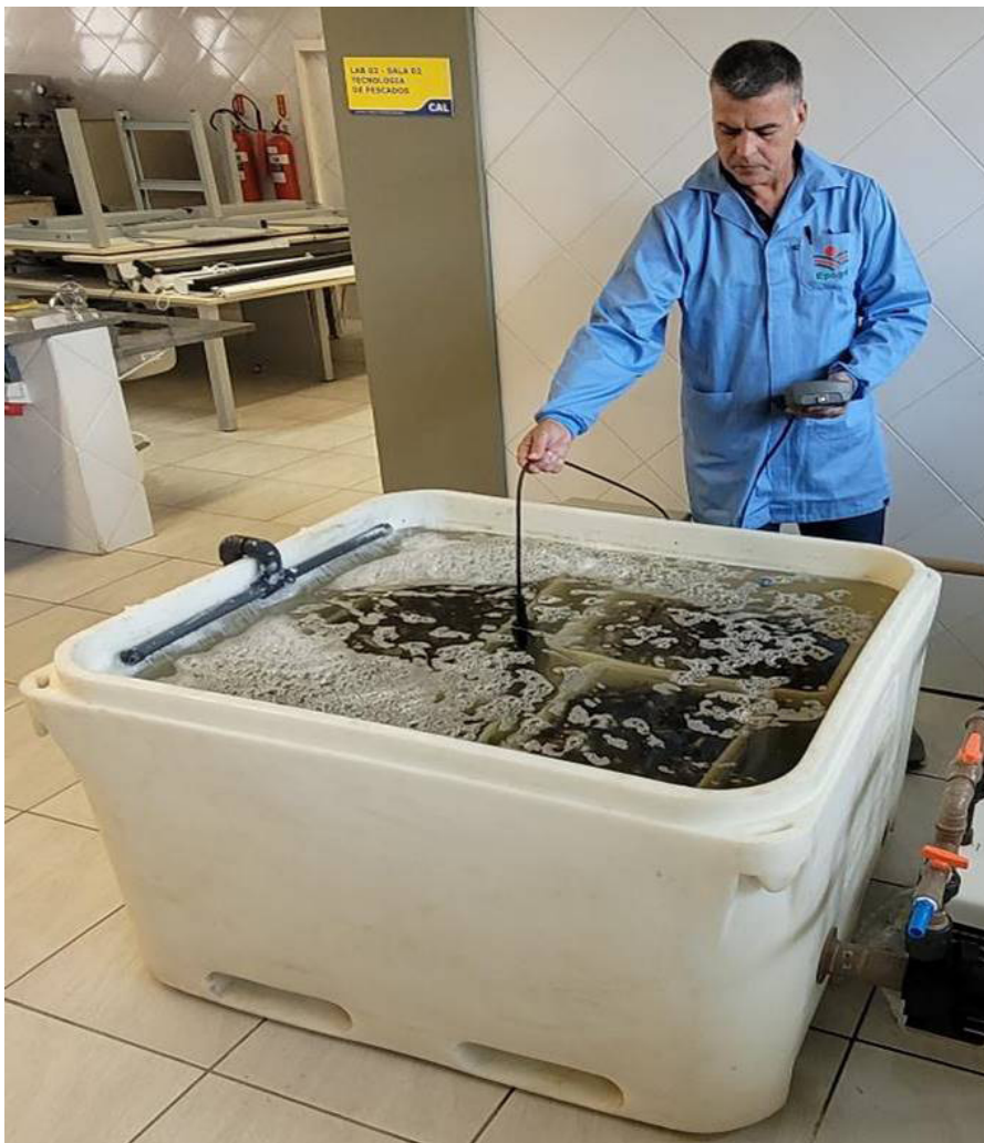
Figure 1. Small-scale deputation unit used in the study. The unit was composed of a 600L deputation tank and a recirculation system containing a water pump, a chiller, and an ultraviolet sterilizer
