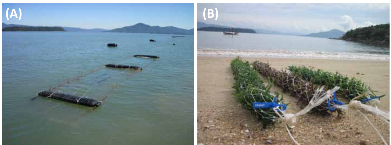
Figure 5. Field tests with the new elliptical flotation model. (A) Culture rafts spaced 5 m, with double long lines; (B) Planting of Kappaphycus alvarezii for biomass formation.
