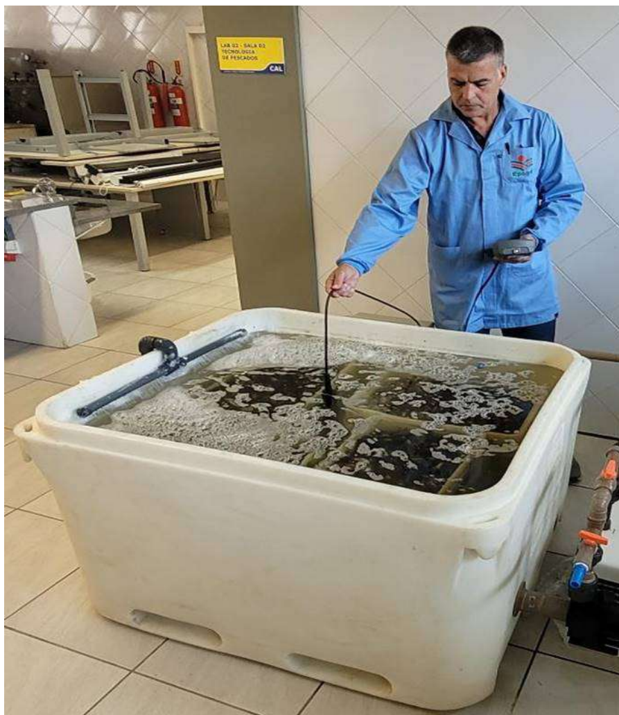
Figure 1. Small-scale depuration unit used in the study. The unit was composed of a 600L depuration tank and a recirculation system containing a water pump, a chiller, and an ultraviolet sterilizer
